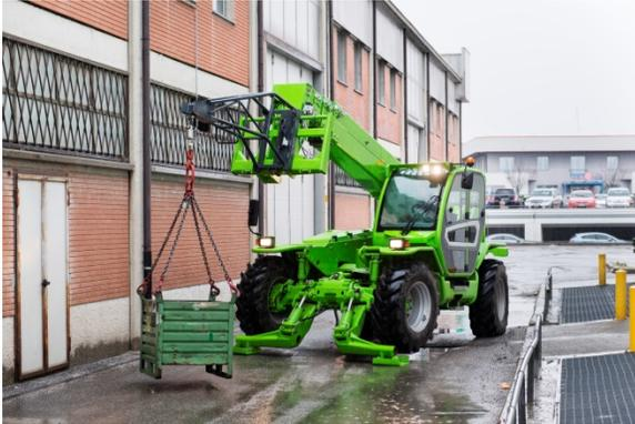
Boom side shift and frame leveling are standard and can be engaged with or without stabilizers in use. Merlo telehandlers are known for their compact footprint and the P50.18Plus is no exception even when stabilizers are deployed. Lighter in mass than similar machines (unloaded weight is 29,300 lbs.) the P50.18Plus offers high ground clearance, hydrostatic transmission,
