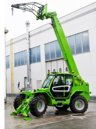
The P50.18Plus is equipped with the Merlo MCDC, a standard operational safety software program. In real time the MCDC automatically recognizes attachments and monitors boom extension, angle, and load weight. Operational options are available to meet specific job requirements.
